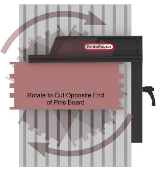
The graphic to the right demonstrates how the reference edges for each board stay against the fence when using this method.
