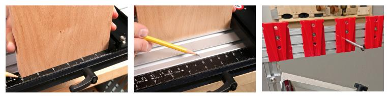
**Check the template and fence location.** For this method to work, it is imperative the centering scale fence is set so the workpiece is accurately centered on the table and the dovetail template sections are laid out symmetrically as described on page 25 of the latest How-To guide.
