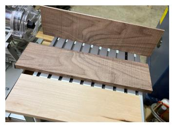
At the band saw, re-saw the drawer front so the thicker inner portion is about 1/32"-1/16" thicker than the desired drawer side dimension.
