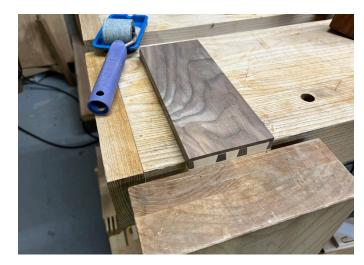
Using a glue roller, apply a light coat to the front of the drawer, you should still be able to see the grain of the wood through the glue. As with a most veneer work, applying the glue to the substrate or in this case drawer front rather than the veneer helps prevent the veneer from warping and makes it easier to work with. If using PVA glue, there is no need to apply glue to both surfaces.
