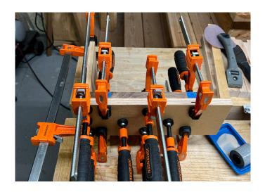
Use a piece of scrap plywood roughly the same dimension as the drawer face as a clamping caul. This task does not require an immense amount of clamping pressure, but rather even pressure across the entire surface area. Using a larger number of clamps with a medium amount of pressure will produce the desired effect while minimizing the likelihood of the false front shifting from the clamping pressure.
