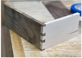
Once all of the tails and pins have been cut, glue up the drawer box. Once the glue is dry, lightly sand the joint so the ends of the tails are not protruding past the drawer face.
