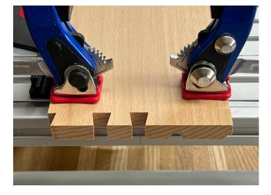
Complete the cut by sliding the router forward again and plunging down from the top of the template slot to remove the remainder of the material.
