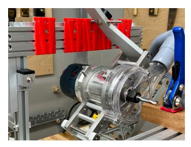
Rather than attempting the cut in a single pass, install a straight bit in the router that is slightly smaller in diameter to the narrowest portion of the finished dovetail cut. In this example, we are using a 3/8" bit.
