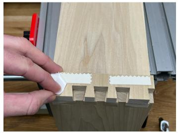
The caul allows clamping pressure to be applied exactly where its needed without interfering with the pins protruding though the tails board resulting in clean closed joints and beautiful through dovetails.
