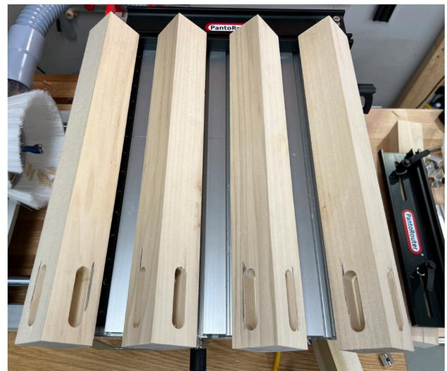
Once all of the mortises are cut in the legs, its time to move on to the tenons.
