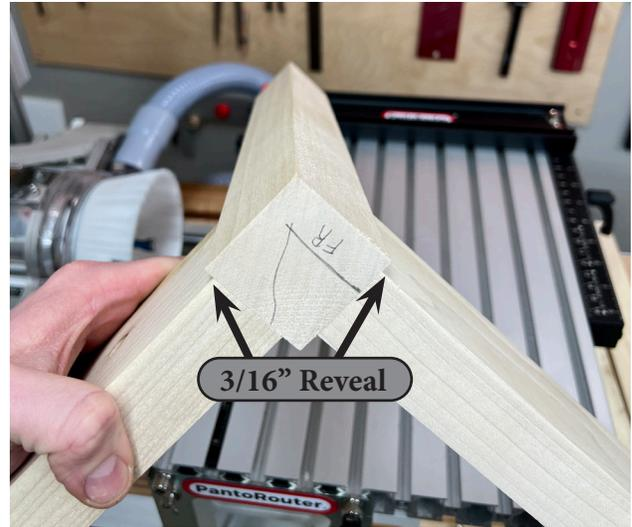
In this example, we created a 3/16" reveal from the face of the leg to the face of the apron. The tenon will be centered in the apron piece but the mortise will not be centered in the leg.
