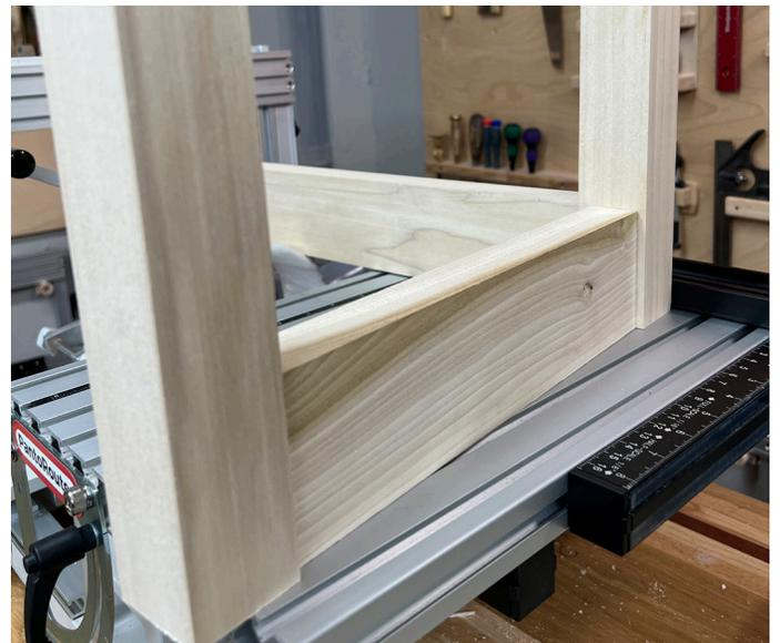
Assemble the table base, and with the legs oriented correctly, there will be a nice consistent reveal on all of the apron and leg joints.
