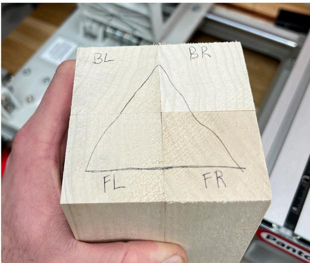
Start by laying out the orientation of the legs and mark them to keep track of outside faces and where the mortises will go.
