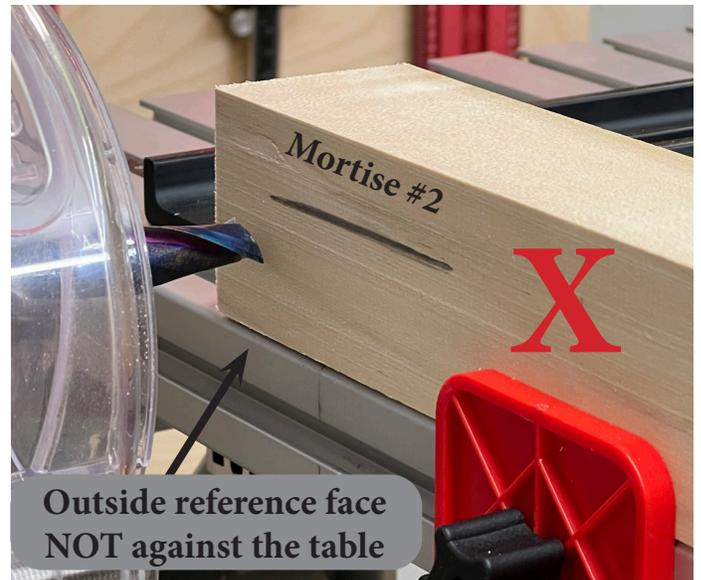
Mark the rough location of the two mortises in each leg with pencil. When the leg is placed on the table and against the Centering Scale Fence, notice that mortise #1 aligns with the bit height but mortise #2 does not. For a consistent reveal, the outside face of each leg needs to be referenced against the table. The issue with mortise #2 is the outside face is not against the table and needs to flip 180 degrees. Each leg will have a mortise #1 and a mortise #2.
