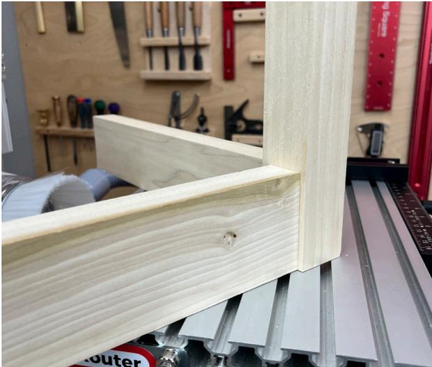
A common detail when joining an apron to a leg of a table is to slightly set the aprons back from the outside faces of the legs to form a reveal rather than making all of the faces flush or centering the aprons in the legs.
