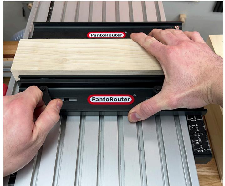
Tighten the lever knobs and then remove the Centering Scale Fence. Now there is a positive stop the same distance from the centerline of the table but on the opposite side. Notice that the Auxiliary Fence does not cover the front table slot so a clamp can still slide in easily .
