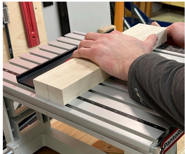
Using the apron stock, set the Centering Scale Fence so the workpiece is centered on the table.
