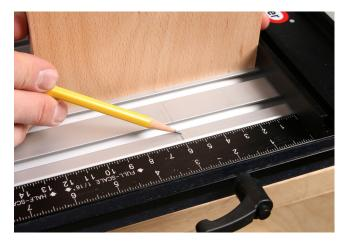
It is critical that the board is accurately centered on the table against the centering scale fence prior to setting the template location with the following method.
