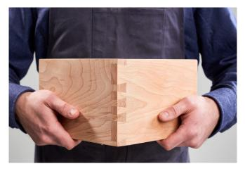
We like the traditional look of a half pin on either end of variably spaced dovetails but it can sometimes be a bit tricky to get them setup perfectly symmetrical.
