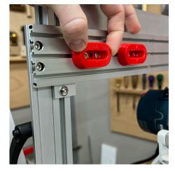
Start with the template holder resting on the thickness gauge and load your templates on, leaving the screws loose enough so the templates can still slide.
