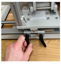
With the Split Shaft Centering Jig pointing towards the markings on the centering bar, lock the front and back depth stops so the PantoRouter carriage cannot move.
